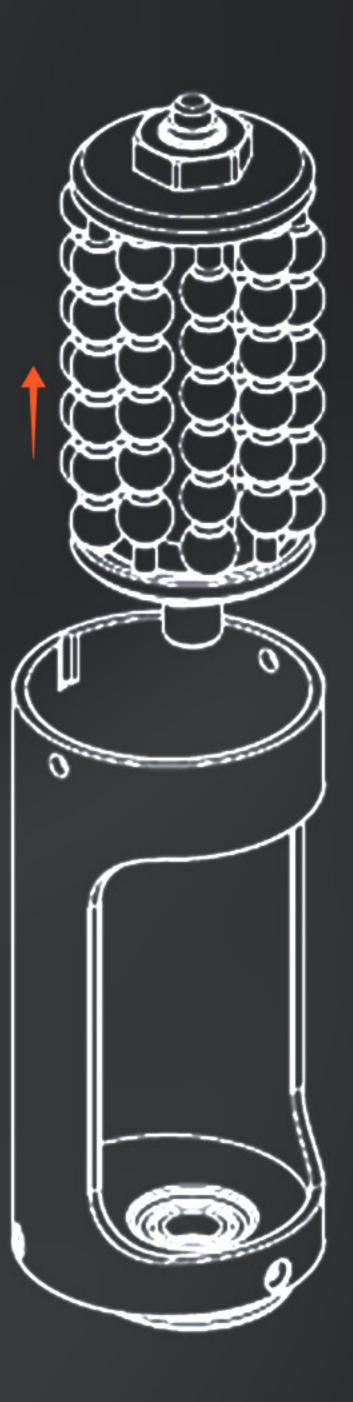
Disassembly and replacement of rotate handle working head:
